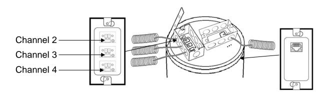
The connection should be made Cat5 or above cable for the Ethernet connection.
