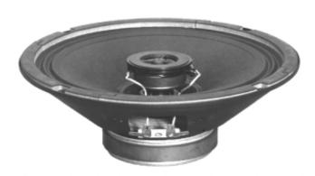
The AMK CX-801 loudspeaker is a full-range co-axial transducer. Its excellent polar dispersion is a result of its high quality polyamide tweeter. This makes it suitable for foreground or background music applications. Most speakers of this type utilize piezo electric tweeters which results in poor off-axis intelligibility. This unit's high efficiency, excellent speech intelligibility, and flat frequency response allow for a wide range of commercial applications.
