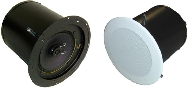
The AMK **SA 801 / SA871** loudspeaker assembly has a full-range, low distortion, and co-axial transducer. Its excellent polar dispersion derived from a high quality broad pattern polyamide tweeter makes it suitable for foreground or background music applications. High efficiency, excellent voice intelligibility, and a smooth high frequency response allow this speaker to be used in a wide range of commercial applications.
